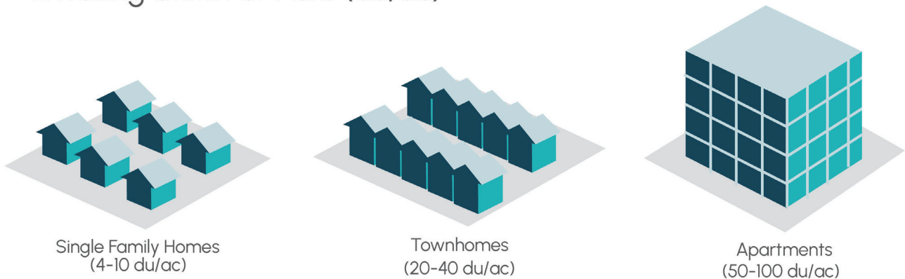
Figure 21: Housing Density and Dwelling Units Per Acre. Source: Civic Results. Derived from Livable Communities Coalition
